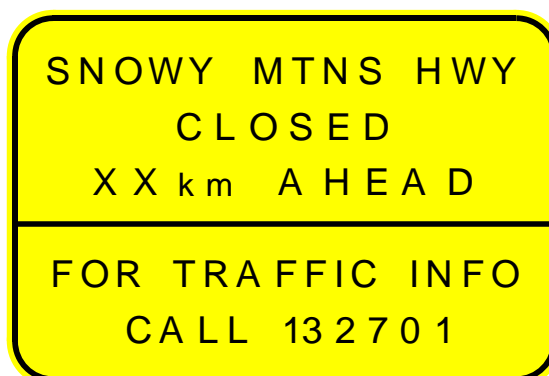
Figure 2 - Advance road closure sign (G9-325-1)
