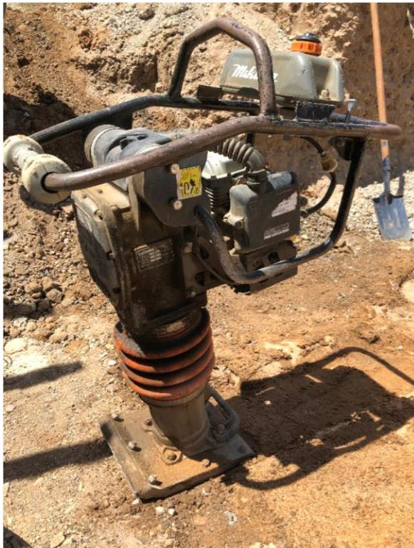
**Figure 3 Wacker Neuson RT82 Trench Roller**
