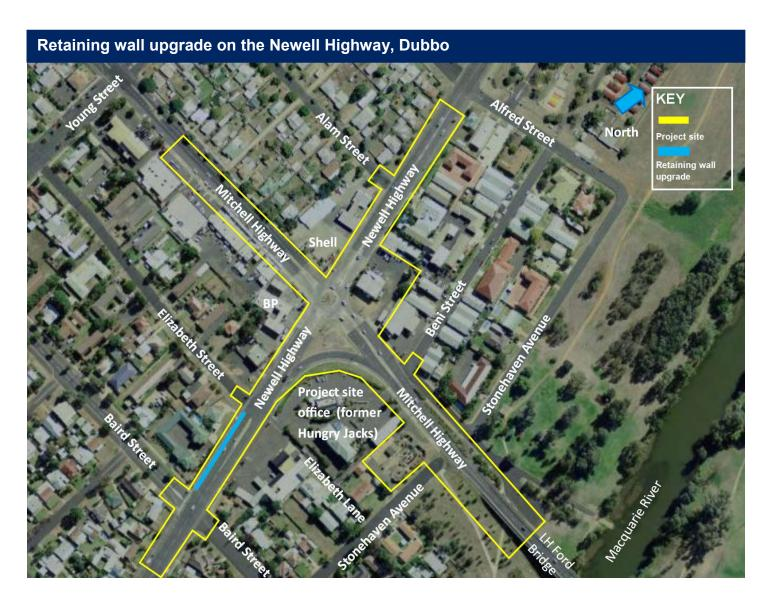
The existing roundabout at the intersection of the Newell Highway and Mitchell Highway will be removed and replaced with traffic lights. The intersection will also be widened as part of the safety improvements.
