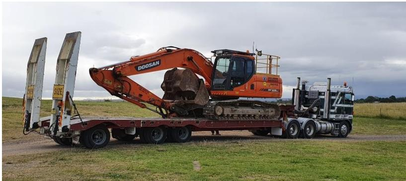
A 20 tonne excavator on a float
