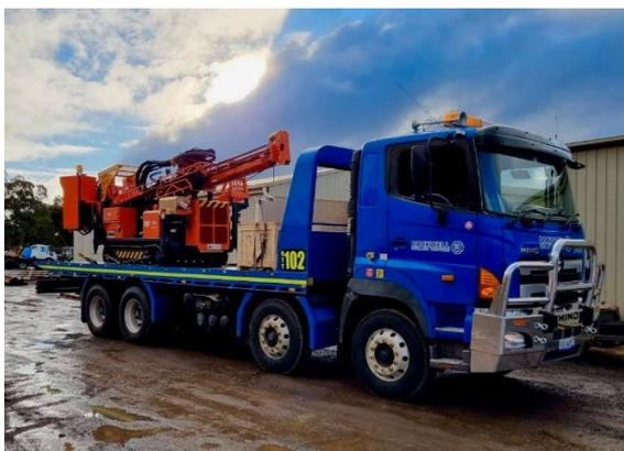
A tracked drill rig floated on the back of a truck
