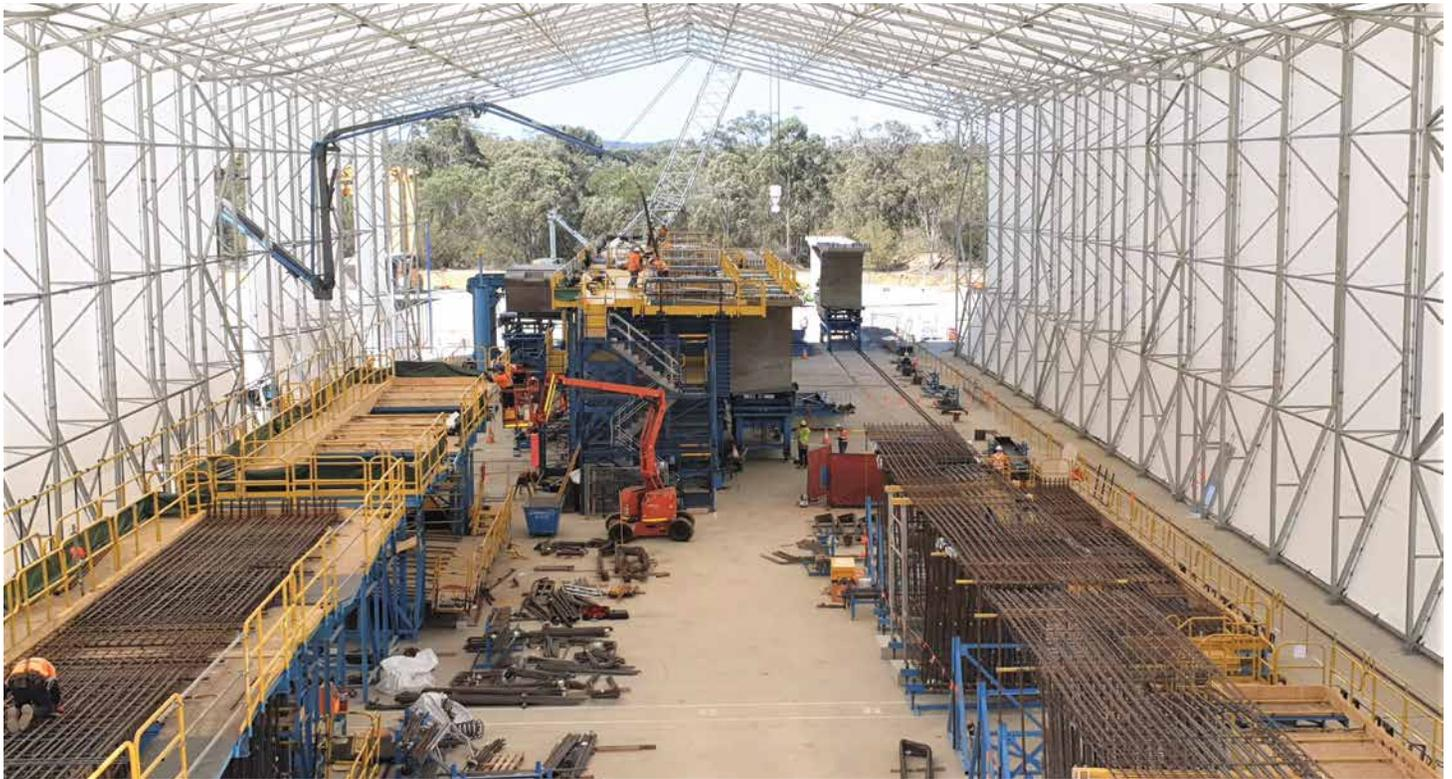
*The interior of the large pre-cast facility shed where all of the concrete segments for bridge construction are produced before they are stored in the adjacent yard and then transported into Batemans Bay.*
