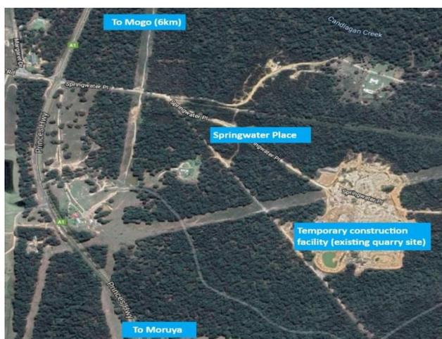
The pre-cast facility is located about 6km south of Mogo in an existing quarry site.
