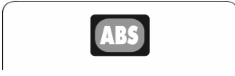
The single lamp is red and indicates the correct functioning of the prime vehicle ABS system and, in some cases, a trailer ABS system.
