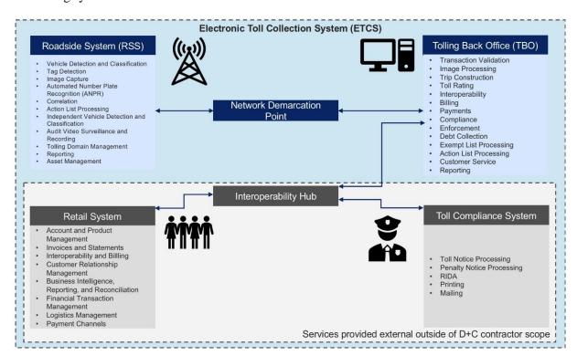
The Electronic Toll Collection System (ETCS) enables the electronic collection of fees for use of Motorway by means of electronic equipment mounted on the roadside and in vehicles.
